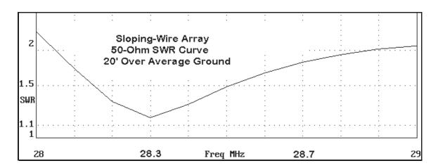
**Figure 3** is the modeled SWR plot across the first MHz of 10 meters. The antenna was designed for 28.35 MHz to provide a low SWR for the most popular segment (28.3 to 28.5 MHz). You can shift the SWR curve downward by increasing the length of both wires equally about 2" or so--or shorten them by the same amount to move a bit up the band. However, keep the wire end separation at the prescribed 9" with the end cross pieces.
