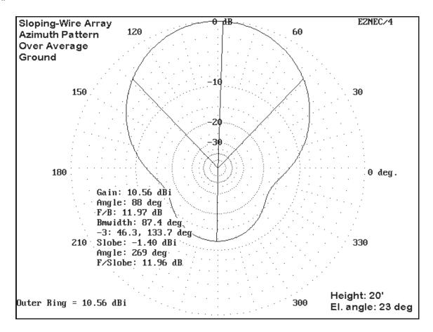
**Figure 2** shows the azimuth pattern with the antenna at 20' over average ground. 20' is the height of two sections of TV masting, which makes an adequate support system for hand rotating the beam. Whatever system you use to elevate the antenna (which I shall assume is as inexpensive as the antenna itself), be certain that the mast is well guyed or bracketed for safety.
