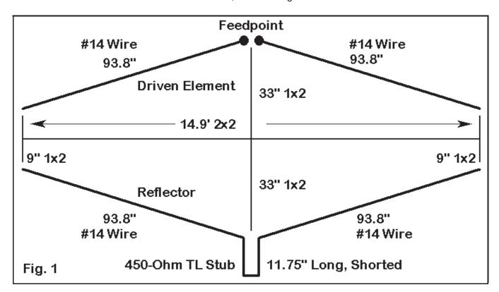
**Figure 1** shows both the wire and support frame dimensions. The 2x2 determines the side-to-side dimensions, while the cross piece determines the maximum front-to-back dimension. The end cross pieces keep the wire ends 9" apart.
